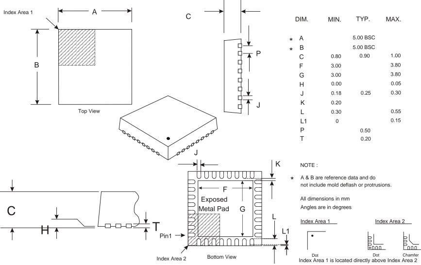
Depending on the method of lead termination at the edge of the package, pull back (L1) may be present.
